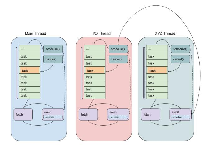
Fig. 2: Lifecycle of a program using multiple pthreads, each running their own threadmaster
