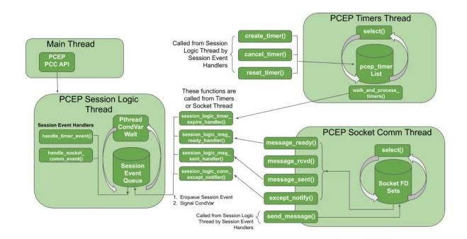
The PCEPlib can also be configured to use an external timers and socket infrastructure like the FRR threads and tasks. In this case, no internal threads are launched for timers and socket comm, as is illustrated in the following diagram.
