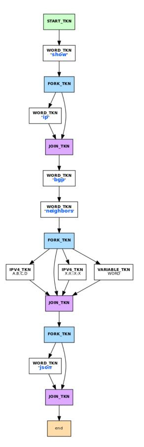
reaches, then the input has matched the corresponding command and the command is executed. If it finds more than one node, then the command is ambiguous (more on this in deduplication). If it cannot exhaust all input, the command is unknown. If it exhausts all input but does not find an edge node, the command is incomplete.
